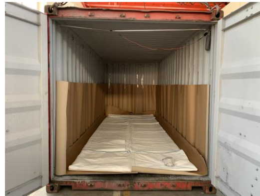
Pic.3 Flexitank installation
