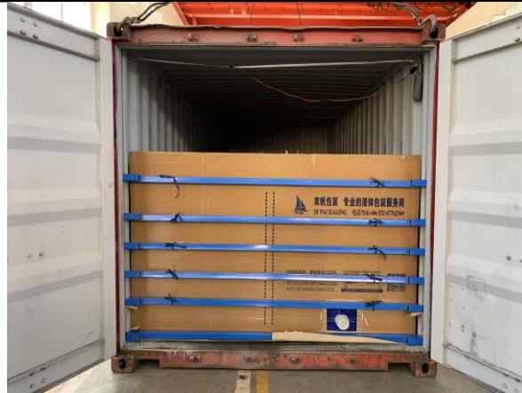
Pic.1 Bulkhead installation
